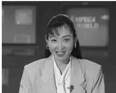
Figure 5-8: Comparison of a frame of “Akiyo”. (a) shows the reconstructed frame with no channel errors, and (b) and (c) show the reconstructed frame after transmission through a simulated GSM channel with 4% BER using (b) EEP coding and (c) UEP coding. UEP produces visibly better images than EEP for the same amount of channel-coding overhead.
